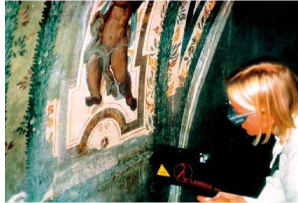
Laser Cleaning of frescoes in the Apostolic Palace of the Lateran in Rome
